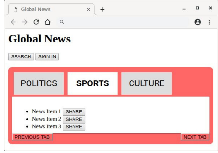
(b) Styling fancy tabs without shadow root affects additionally buttons inside of Fancy Tab.
